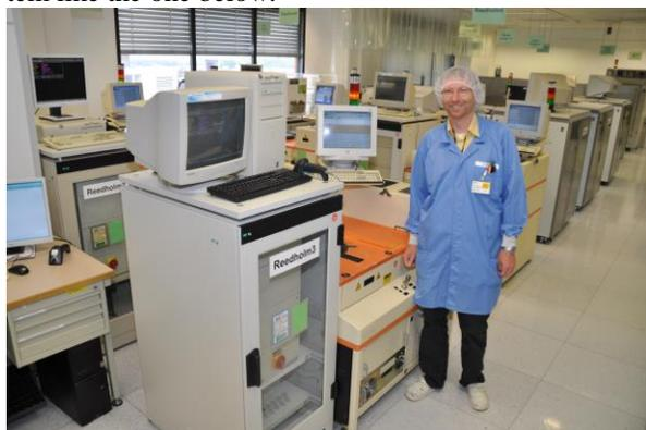
“Empirical values” serve to assess measurement results. If results comply with expectations, the wafer is released to subsequent testing. However, wafers that do not fulfill these expectations are scrapped.
