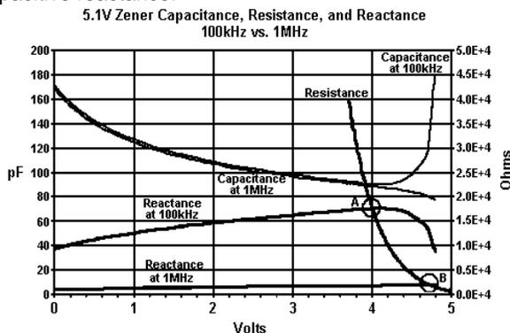
Figure 11 - Zener Diode Capacitance
