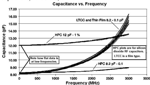
Figure 8 - Silicon Oxide Capacitance vs. Frequency
