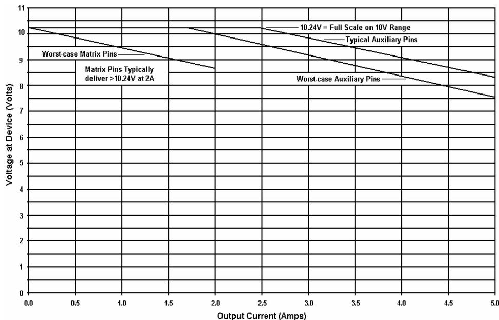
Figure 3 - Voltage Delivery in RI-2kV/5A Test System
