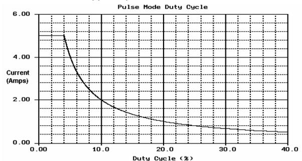
Figure 2 - Duty Cycle and Output Current
