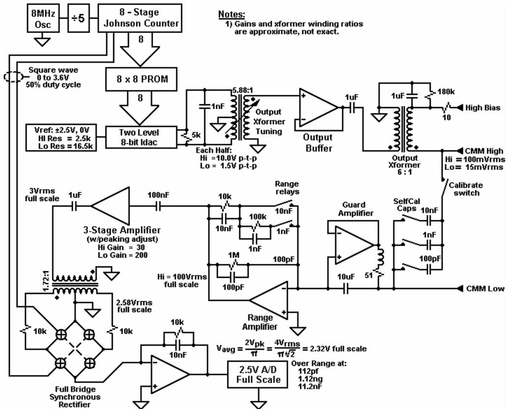
Figure 2 - Simplified Schematic of 100kHz CMM
