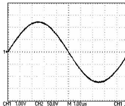
Figure 5 - DAC Output at Tuned Transformer
