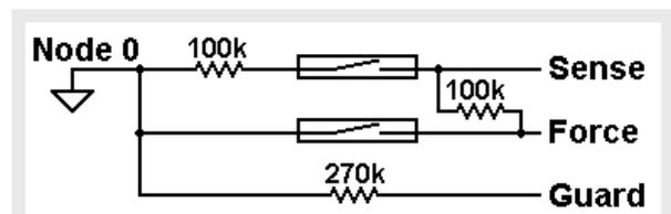
Resistance added to the node 0 sense path prevents welding of the sense relay, but provides a discharge path if there is voltage present. The force relay is not allowed to close until voltage is  $<|1V|$ , which is below the arcing voltage. Thus, even if there is switch bounce, the voltage is too low to transfer material, which leads to welding, or sticking, of contacts.
