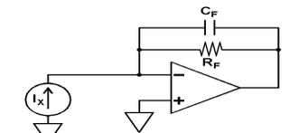
Figure 4 - Feedback Ammeter
